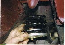
The top arm can then be refitted by replacing all the components in the reverse order to which they were removed, remembering to clean them first. The new coil and seat can then be inserted.
