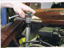
There are two types of threaded bar on spring compressors, so make sure you have the correct one. Screw the inner section into the rubber cone, making sure it goes all the way in to prevent it pulling out when under pressure.
