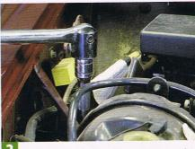
With the car jacked up and safely supported on some axle stands, remove the road wheels. Next, undo the large tower bolt using a large 1 5/16 AF socket. You may find it makes it easier if you remove the bonnet as well.
