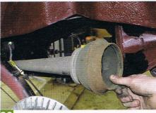
You will need to remove the rear damper and then push the suspension arm down as far as it will go. This will allow you to remove the rubber cone and trumpet. They may need prising out with a large screwdriver or something similar.
