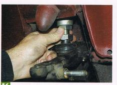
We set the Hi-Los at a midway point and loosely wound up the locking nut. If you removed the top ball joint then this will also need reassembling and tightening to 40lb.ft using a torque wrench and 11/16-inch AF socket.
