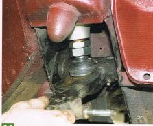
Next insert the new Hi-Lo adjuster - at the moment you will just have to guess the correct adjustment as this will need setting up properly once all four corners are completed.
