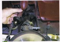
By pushing the suspension fully down you should now be able to remove the suspension trumpet - these may need a little bit of persuading to get them to release from their seats. With the trumpet removed, you can now release the tension on the rubber cone.
