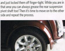
After each adjustment, replace the wheel, push the car back and forth a few times and then check the ride height again. You may find further settlement over time, but once you're happy with the ride height make sure you tighten the nut on the Hi-Lo.
