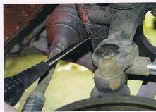
The lower rebound rubber will also need to be removed. For this you will probably need to clean off the small crosshead screw that holds it in place and then undo it with a suitable screwdriver.
