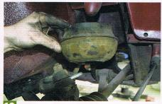
Remove the large washer and seal and then withdraw the pivot shaft. The top suspension arm can now be removed to allow you to lift out the rubber cone. At this point we found that the plastic cup needed replacing and so we needed to release the top ball joint with a suitable ball joint splitter.
