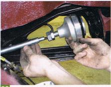
You can then fit the rest of the Hi-Lo, the spring and its seat in the order shown. Following this you will need to raise the suspension arm to hold it all in place. Use a jack or similar to hold it up.
