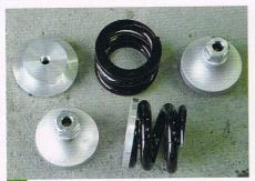
New coil springs and adjustable ride height kits are available from most Mini specialists. The coils simply replace the standard rubber cones and come in various configurations for road, fast road and track use.
