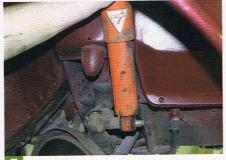
Moving to under the arch, you can now undo and remove the front damper by removing the nuts and large washers holding them in place and then sliding it off the locating pins.
