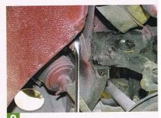
To get the cone out you will need to remove the top suspension arm. Start by undoing the nuts at either end of the pivot shaft using a 3/4-inch AF spanner, and then remove the retaining plate that prevents the shaft from coming out.
