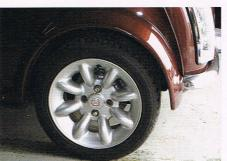
A good way to check the ride height - with the car on level ground - is to measure the distance between the ground and the sill at points as close to each wheel as possible. This should ensure that the car sits level.
