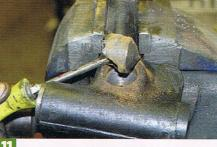
With the arm removed from the car we were able to mount it securely in a vice so that we could prise out the old plastic cup using a screwdriver. It is possible to do this insitu so you don't have to remove the top arm completely - it all depends on how easily the cup comes out.
