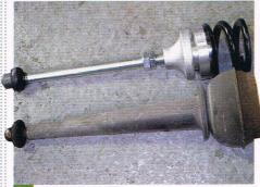
Repeat for the other front wheel and you can then start on the rear. Here you can see a standard rear trumpet and rubber cone next to the replacement coil spring, seat and Hi-Lo.
