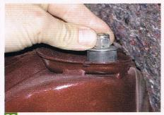
With everything in place you can then refit the rear damper to the radius arm and up through the hole in the suspension tower. The top nuts can then be fitted back on and the petrol tank strapped back in on the near side.
