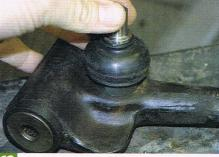
The new knuckle joint we used came complete with a new plastic seat, so this was duly fitted to the top arm. If the existing seat is still serviceable and you are retaining the old knuckle joint then simply clean and re-grease it and then fit back together.
