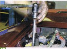
The tower bolt will also need to be refitted at this point using your large 1-5/16-inch AF socket, extension bar and T bar or similar. Make sure the tower bolt is tightened fully to prevent any possible movement of the subframe.
