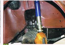
The damper unit can also be refitted and should keep everything together while you fit the road wheel and get the car back on the ground. If you plan to lower your car then you might want to consider dampers designed for lowered Minis.
