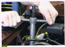
Next, turn the 'T-handle', which will draw up the inner section, thus compressing the rubber cone. This can become quite stiff so you may need to use a short extension bar to increase the leverage.
