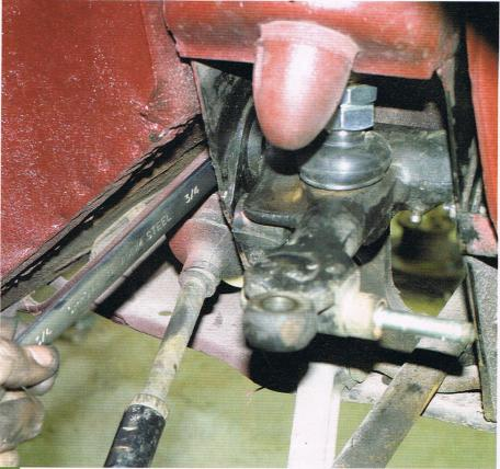
You can now fit the nuts and washers back onto the pivot pin and then install the locking plate, making sure everything is done up tight. A good
